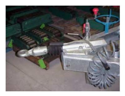
The British eyeshafts have a round or toroidal section eye and are used with a parallel type pin with sufficient clearance in the eye to permit the correct sequence of towing on the pin and braking on the jaw. If the pin is too large or the clearance between the jaw and pin too great, then both towing and braking loads will be put onto the pin.
